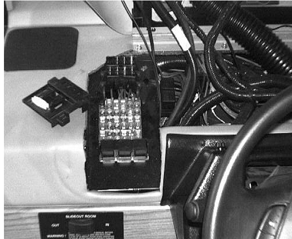
Automotive 12-Volt Fuse Panel Beneath Lift-Up Dash Pod
