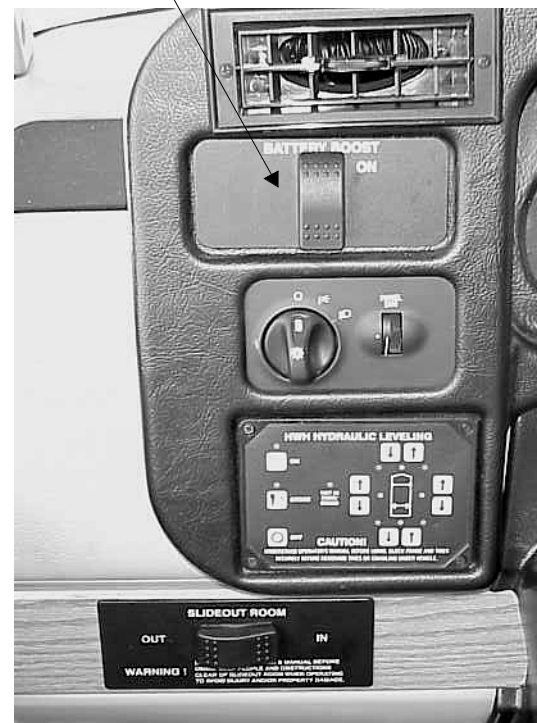
Battery Boost Switch
