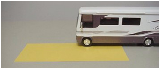
Weighing Left Front 'Corner'
