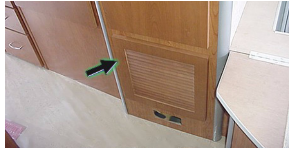
Carefully pry panel from lower face of wardrobe cabinet using thin blade-type tool.
