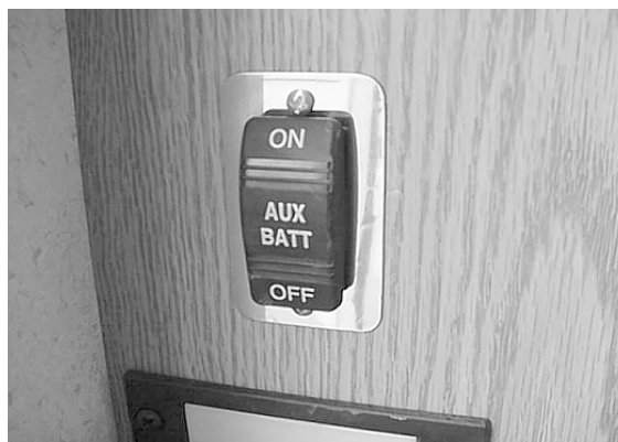
Aux. Batt. Disconnect Switch Model 23H - on back side of dinette Model 23J - on end of galley
