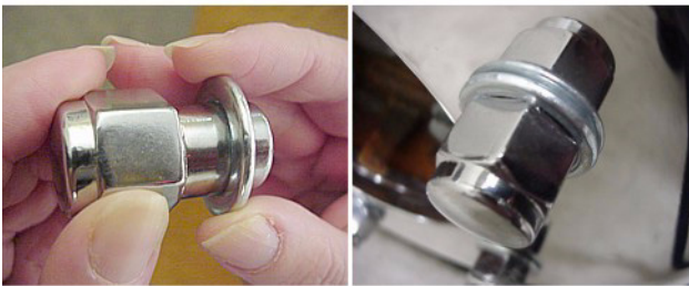
Aluminum Wheel Lug Nut and Washer (Extended Thread Shoulder Nut)
