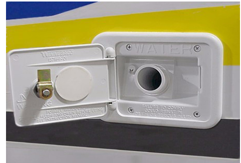
Water Tank Gravity Fill
