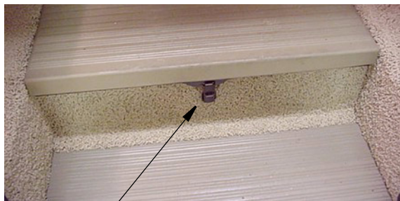
Release latch and lift step to access house and chassis batteries
