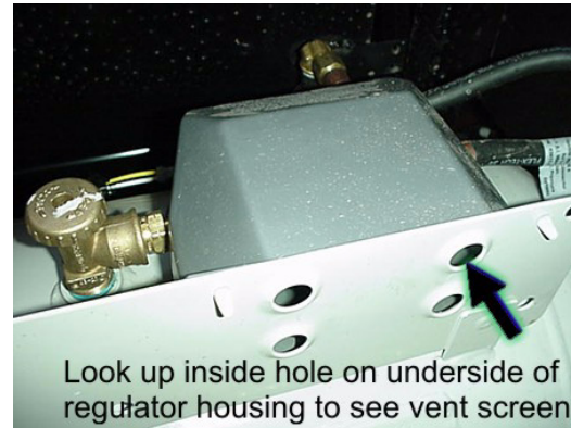
LP Gas Regulators (additional one on top is for LP fueled aux. generator if equipped)
