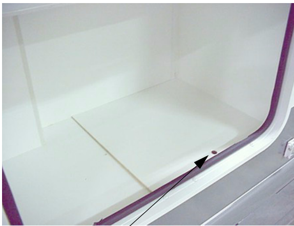
Finger hole - Lift panel to access pump, strainer, drain valves and winterization valve.
