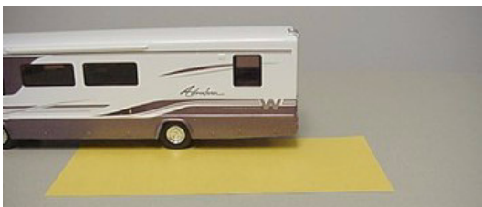
Weighing Left Rear 'Corner'
