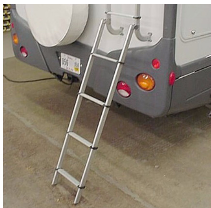
Pull pin to lower ladder extension
