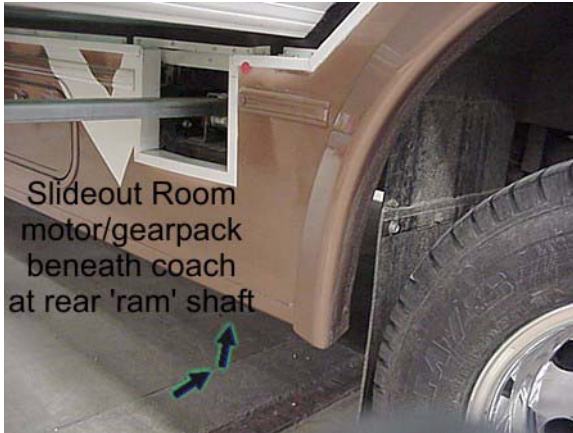
Slideout Room motor/gearpack beneath coach at rear 'ram' shaft Front Slideout Motor/Gear Location beneath driver side of vehicle All Models
