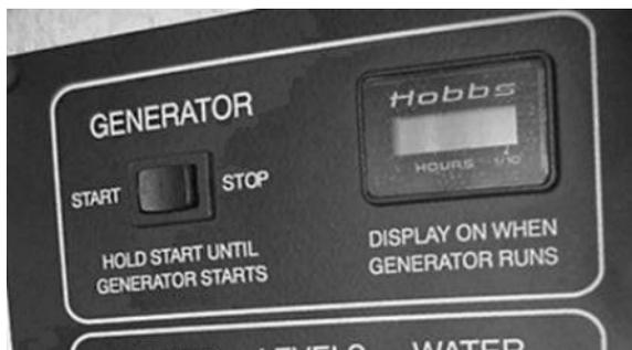
Refer to the hourmeter to determine when periodic maintenance is due and to record services which have been performed.
