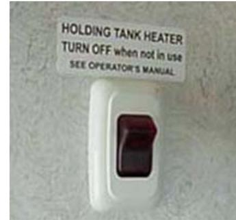
DO NOT operate the holding tank heater unless you are providing a supplemental 12-volt power source to recharge the house batteries. This means either the shoreline cord must be plugged into a 120-volt source, or the auxiliary generator must be operating, or the chassis engine must be running (such as when driving down the road). This will prevent excessive discharge of the house battery.
