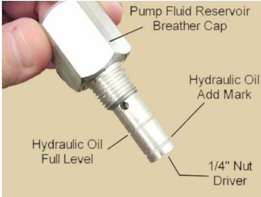
*NOTE: Overfilling the hydraulic reservoir can cause leakage of oil through the breather cap.*
