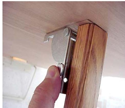
2. Remove the table from the wall support bracket by lifting the end of the table. Then lower the table to rest on the cleats attached to each dinette bench.
