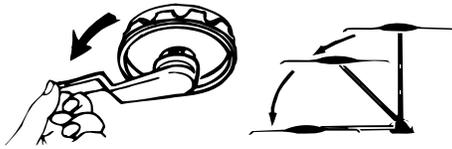
Turn elevating crank (counterclockwise) in “DOWN” direction until resistance is noted (about 13 turns). Antenna is now locked in travel position. Turn amplifier power switch “OFF”.
