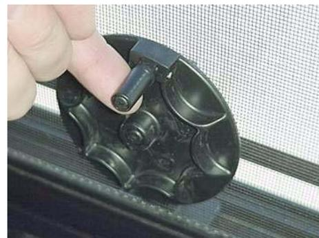
If the window will not open after three or more full turns of the knob, the glass may be stuck to the sealing gasket. Go to the outside of the coach
