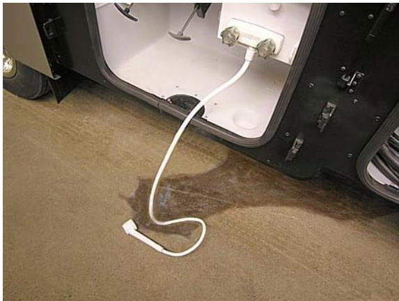
Using exterior shower to drain water line
