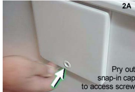
**Type B–Single Arm – Cover mounted beneath face of slideout room:**
