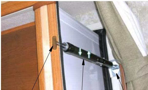
Place T-shaped rod end against back side of slideout frame      Rotate cylinder body to loosen or tighten ends      Place flat plate end against coach sidewall
