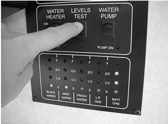
The approximate fluid levels are measured by electronic sensors on the sides of the tanks. There is generally more fluid in a tank than indicated on the monitor panel.
