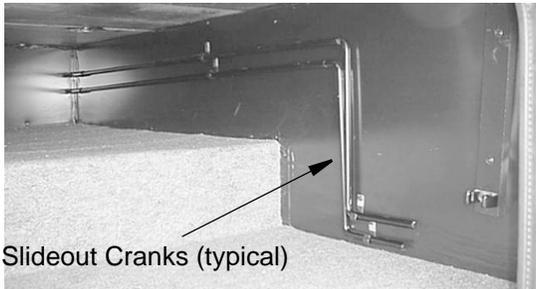
The crank sockets are located behind covers on the lower ends of the room on the outside of the coach. Your coach may have one of the two types of covers shown.
