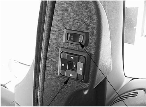
**Mirror Adjustment Control      Mirror Heat Switch**
