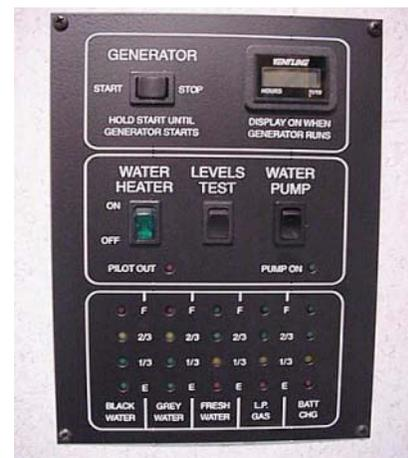
At the touch of a button this panel will display the fresh water and holding tank levels, propane gas tank level, plus the house battery condition. You can start the generator or turn on the water pump and water heater. Indicator lights tell you if the water pump is on or if the water heater pilot light is out.
