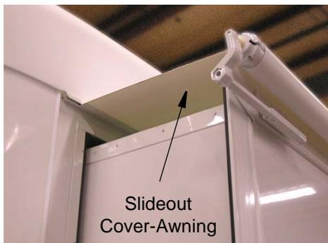
Also, freezing rain and snow can prevent the slideout cover-awning (if equipped) from closing and may cause damage to the cover-awning, slideout room, weather seals and mechanisms.
