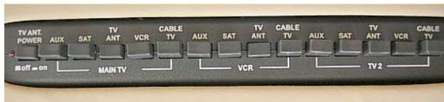
The video selection system allows you to switch the antenna, cable TV, satellite TV system or VCR/DVD signal to any TV set location in the coach.
