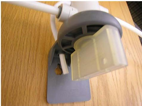
2. Remove the filter canister from the full-coach water filtration system in the water center compartment (if equipped) and discard the filter cartridge. *(If your coach is not equipped with a full-coach water filtration system, proceed to the next numbered step.)* After removing filter, remount the empty canister onto the filter assembly and continue the antifreeze fill procedure.
