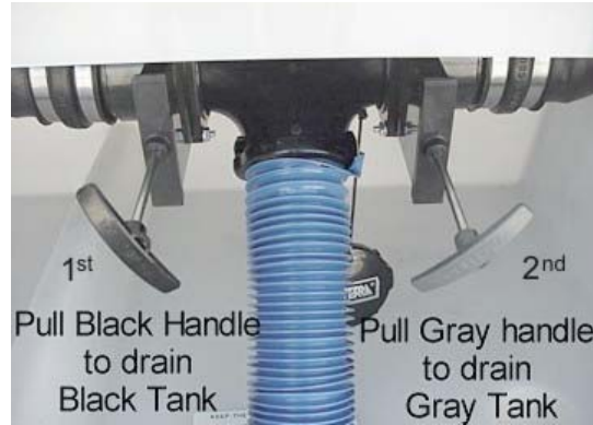
Holding Tank Dump Valves (Typical)
