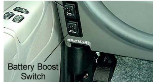
Battery Boost Switch
