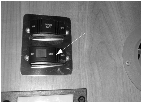
Entry Step Switch (Located near entrance door)
