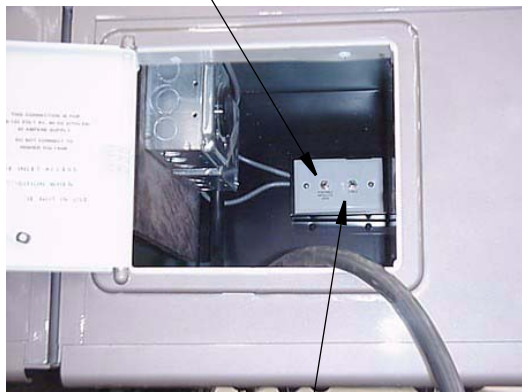
Portable Satellite Dish Hook-up in Shoreline Compartment
