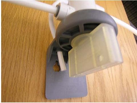
Diverter Plug installed in filter socket. Insert and twist 1/4-turn clockwise (to the right), same as filter installation.
