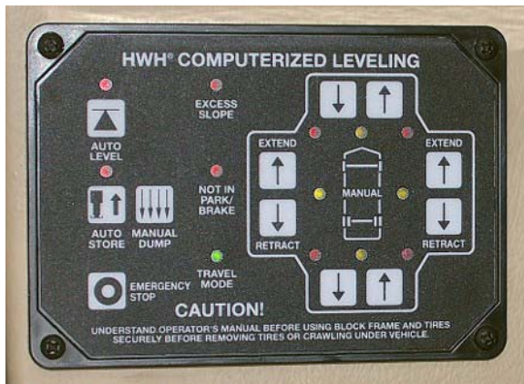
Leveling System Control Panel
