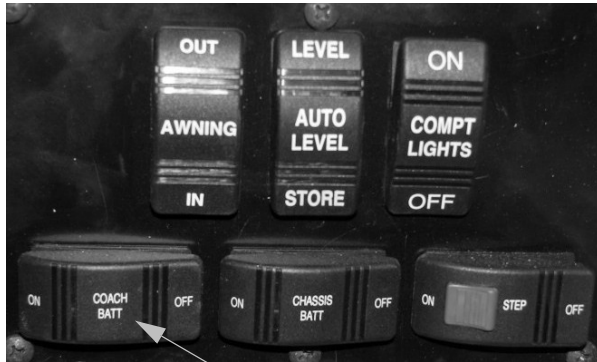
Auxiliary Battery Switch - Typical (Near Entrance Door)
