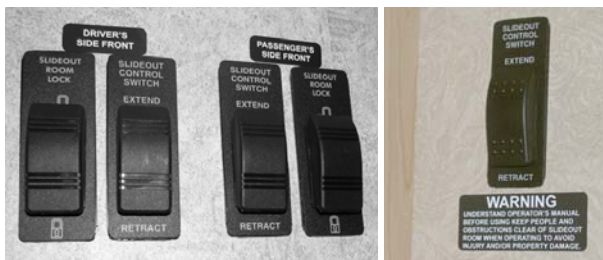
Slideout Room Locks and Switches (Your model may be equipped with one or more types) -Typical View
