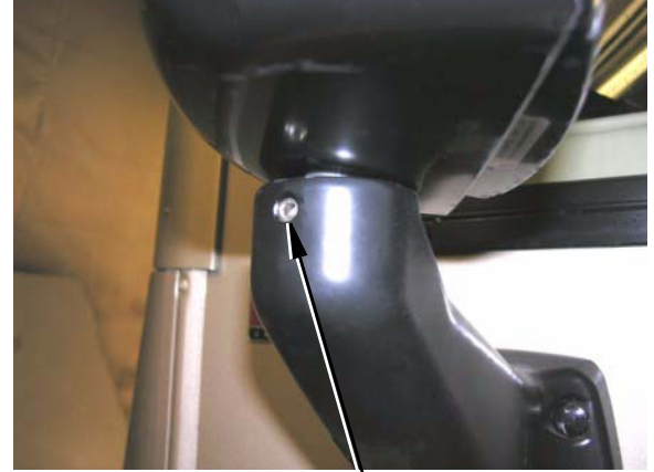
Mirror Head Pivot Lock Loosen Allen head set screw to pivot mirror head.* (Torque 75-100 in/lbs)
