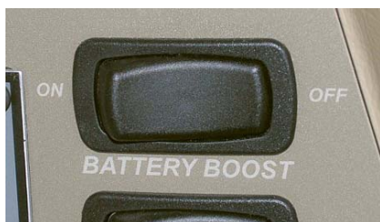
Battery Boost Switch (located on dash)
