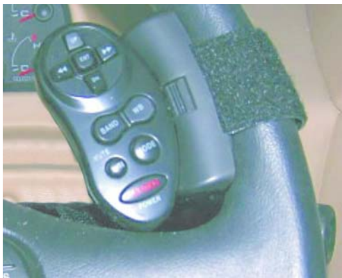
Radio Remote Control (Ford® Chassis) -Typical View
