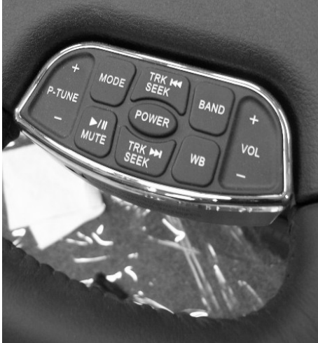
Radio Remote Control (Workhorse™ Chassis) -Typical View
