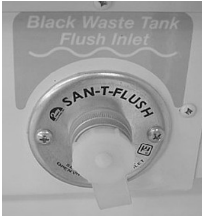
Black Water Tank Flush Inlet (Located in water service center) -Typical View
