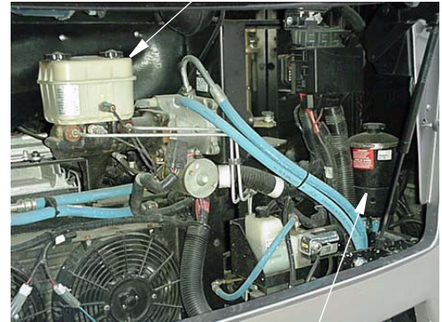
Power Steering Fluid Reservoir Driver Side - Typical View
