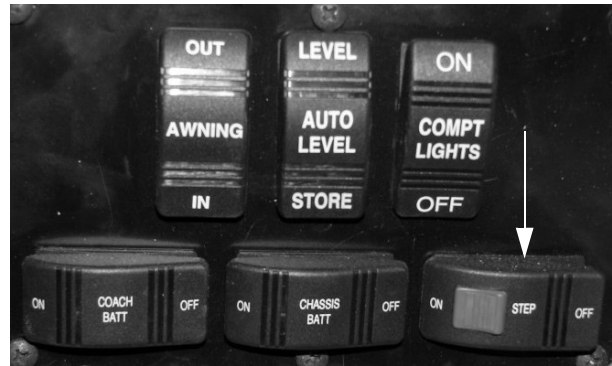
Entry Step Switch - Typical (Located near the entrance door)
