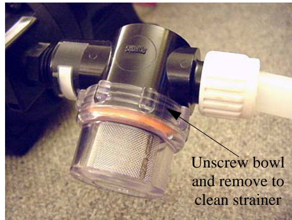
Water Pump Strainer -Typical View
