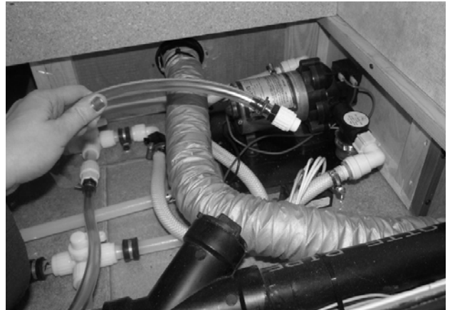
RV Antifreeze Siphon Tube (Located near water pump) * Insert into container of RV water system antifreeze
