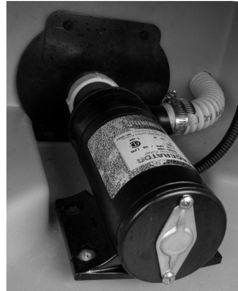
Waste Pump (Located underneath the rear driver side of coach) -Typical View
