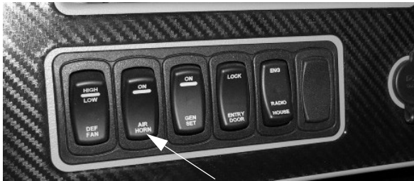
Air Horn Switch (Located on dash) -Typical View
