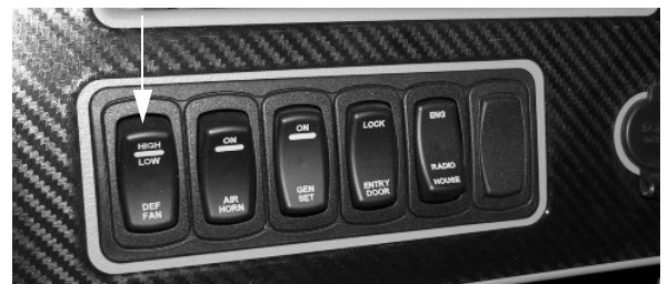
Defrost Fan Switch (Located on dash) -Typical View
