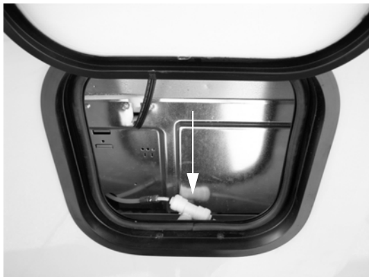
Ice Maker Winterization Drain Valve (Located behind sidewall access door) -Typical View
