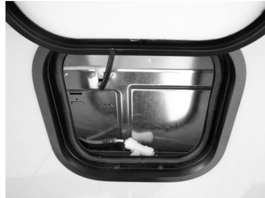
Residential Refrigerator Access Compartment -Typical View
