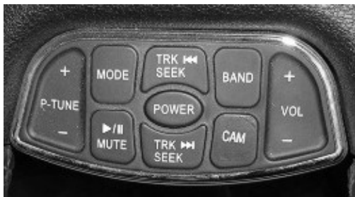
Steering Wheel Radio Remote Control
