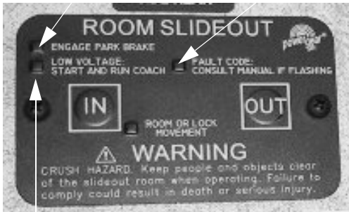
Slideout Touchpad (Located near monitor panel) -Typical View
