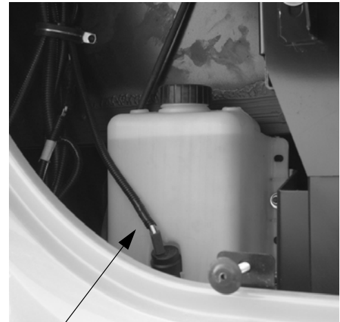
Windshield Washer Reservoir (behind front hood panel)
