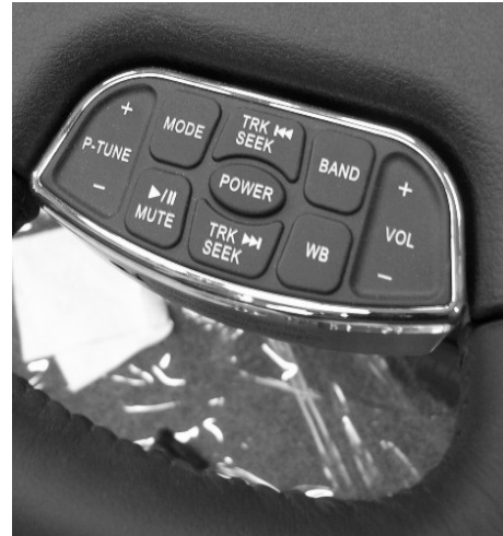
Steering Wheel Radio Remote Control
