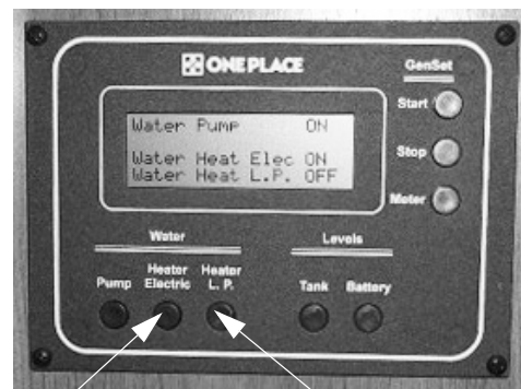
Electric Water Heater Switch LP Gas Water Heater Switch
