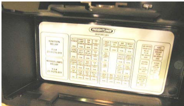
Fuse Diagram (inside of cover)
