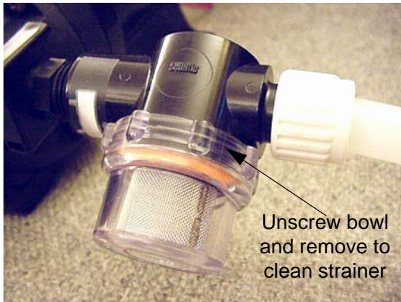
Water Pump Strainer -Typical View
