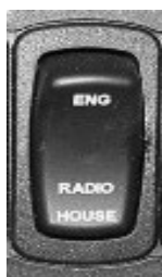
Radio Power Switch (Located on dash)
