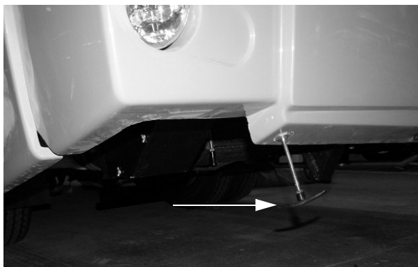
Gray Waste Tank Drain Valve (Located underneath rear driver side bumper)
