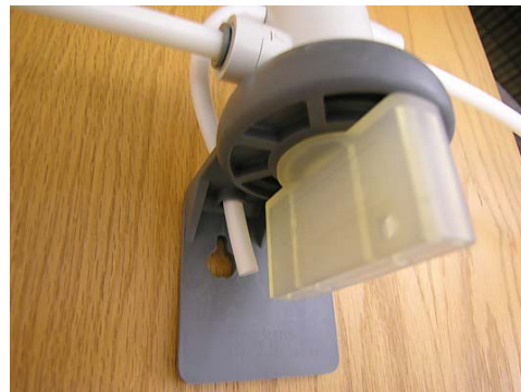
Diverter Plug installed in filter socket • Insert and twist 1/4-turn clockwise (to the right)
