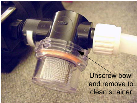
Water Pump Strainer -Typical View
