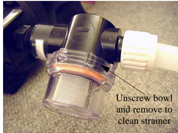
Water Pump Strainer -Typical View
