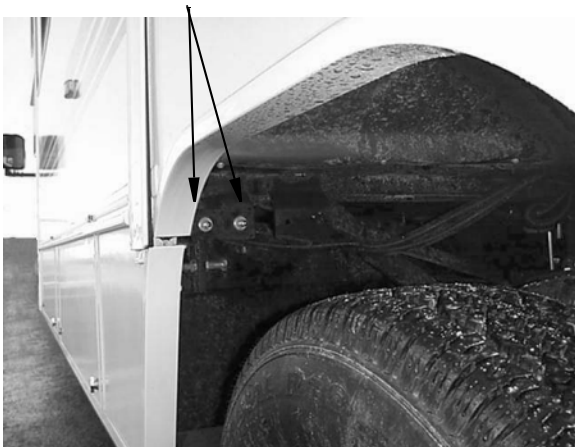
Rear Air Spring Valves (Located inside left rear wheel well -Typical View
