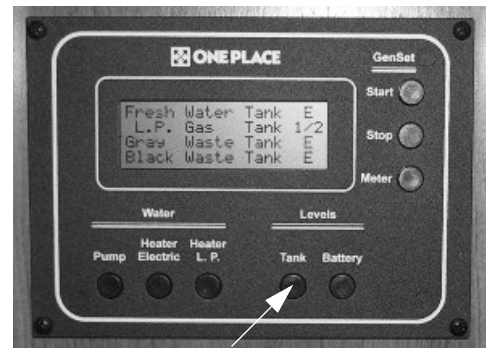
Tank Levels Switch
