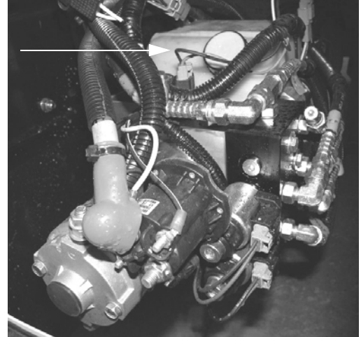
Hydraulic Oil Reservoir (Located behind driver side front tire) -Typical View
