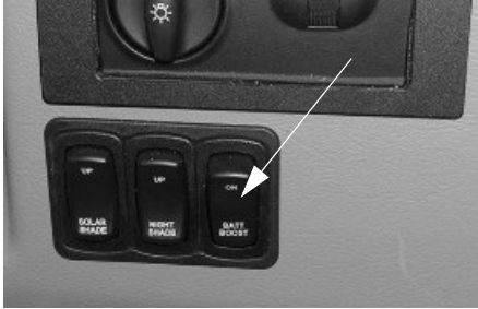
Battery Boost Switch (Located on dash)
