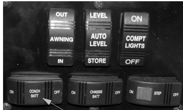
House/Coach Battery Disconnect Switch (Located near entrance door) -Typical View
