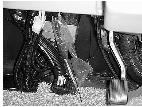
CB Power Wires (in plastic sheath)
