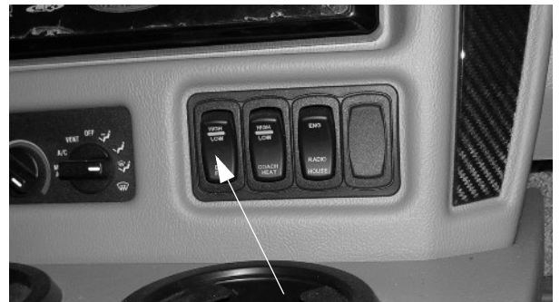
Defrost Fan Switch -Typical View
