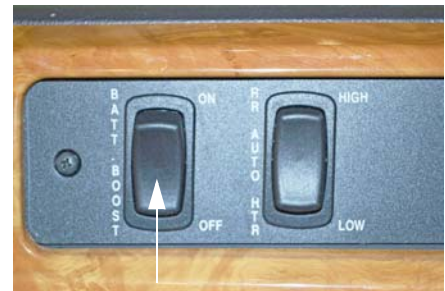
Battery Boost Switch
