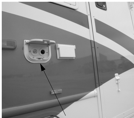
Exterior Cable TV / 12-Volt Connection (Located near entrance door) -Typical View
