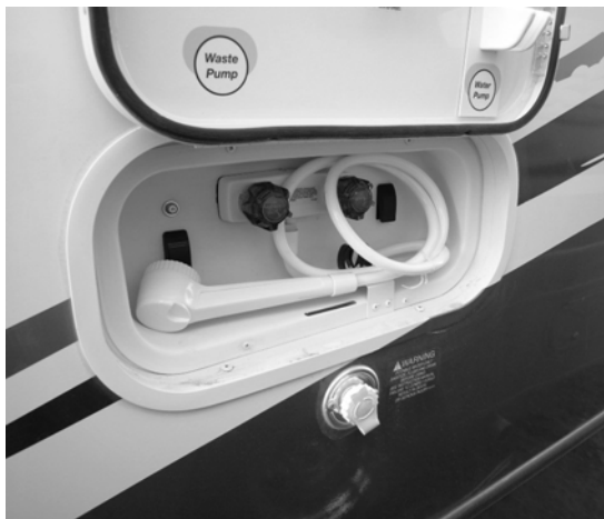
Exterior Shower/Wash Station -Typical View
