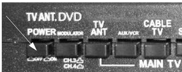
TV Signal Amplifier Switch (Located on Video Selection System)
