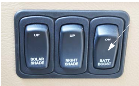
Battery Boost Switch (Located on dash)
