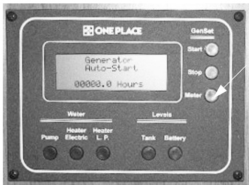
Generator Hourmeter Button -Typical View
