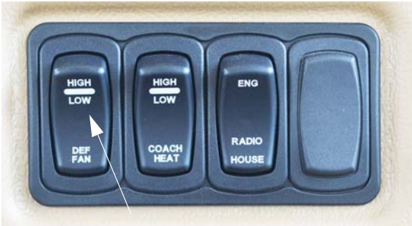
Defrost Fan Switch -Typical View
