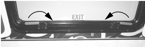
Escape Window (Lift both red safety latch handles UP and push window OUT) -Typical View
