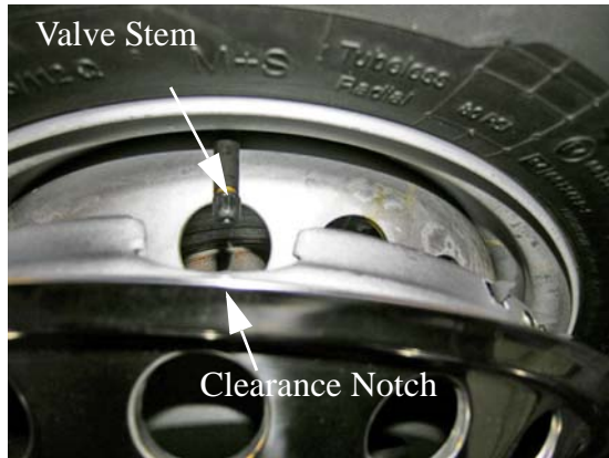
Valve Stem Clearance Notch aligned to Valve Stem
