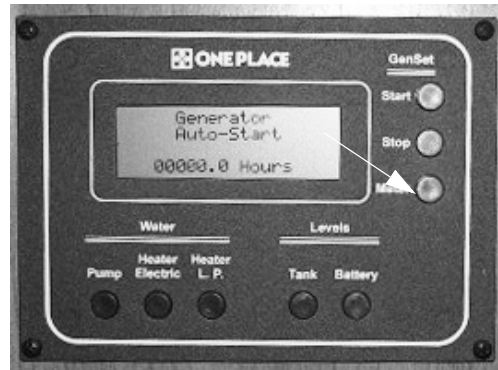
Generator Hourmeter Button -Typical View
