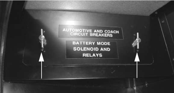
Automotive Chassis and House 12-Volt Circuit Breakers (Located in passenger side compartment) * Turn latches to remove cover
