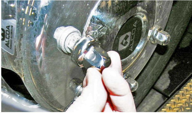
Remove the push on nut covers.
