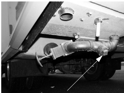
Waste Pump Drain (Located underneath rear driver side of coach) * Models 25T and 25Q only
