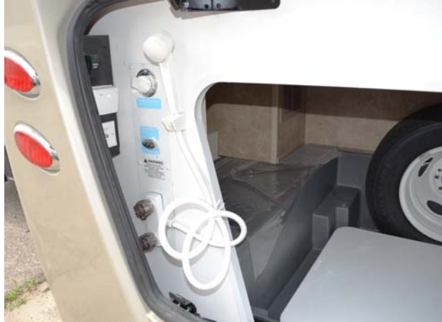
Using exterior shower to drain waterline.
