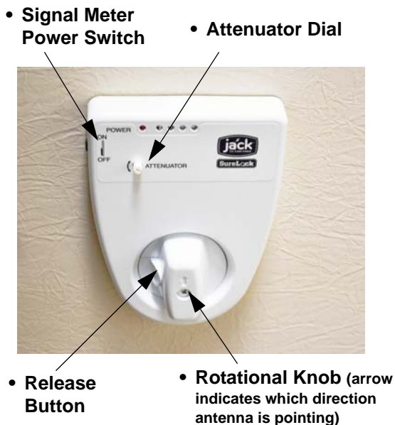
Digital Antenna Signal Meter (Located on ceiling)
