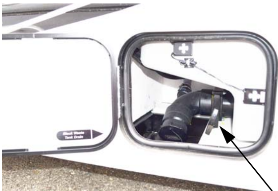
Black Waste Tank Drain Valve (Located in driver side compartment ahead of rear wheel)
