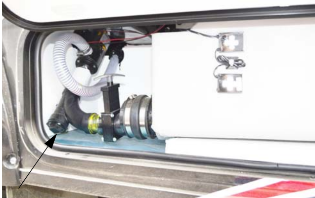
Waste Pump Drain (Located in driver side compartment behind rear wheel)
