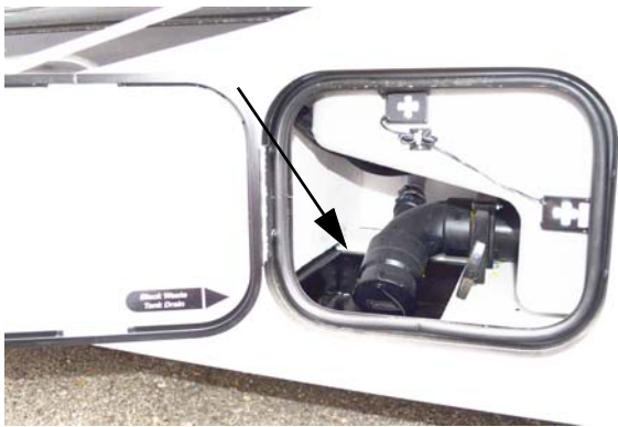
Sewage Drain Outlet (Located in driver side compartment ahead of rear wheel)
