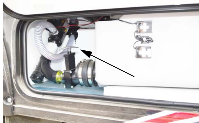
Gray Waste Tank Drain Valve (Located in driver side compartment behind rear wheel)
