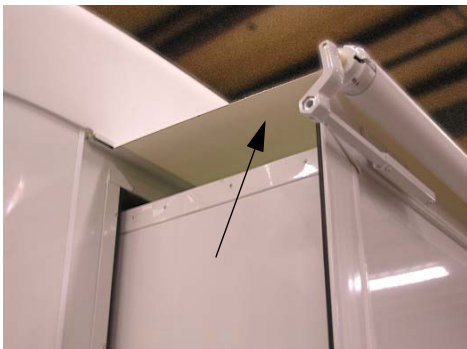
Slideout Cover-Awning -Typical View
