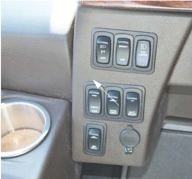
Battery Boost Switch (Located on dash)
