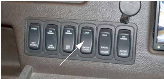
Power Door Locks - Entry Door (Located on dash) -Typical View
