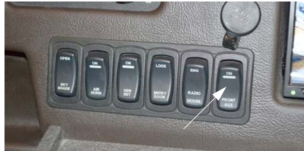
Front AUX Switch (Located on dash) -Typical View
