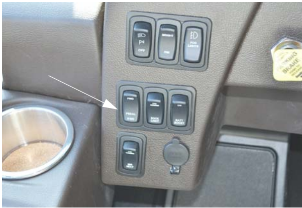
Adjustable Pedal Switch (Located on dash) -Typical View
