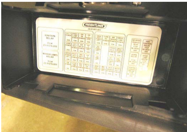
Fuse Diagram (inside of cover)
