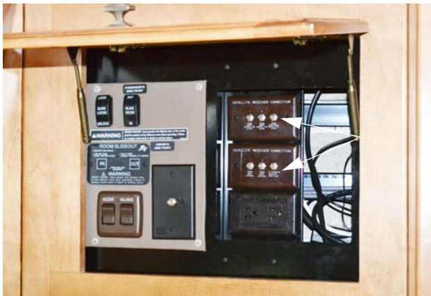
Interior Connections for Satellite Dish (Located in the overhead compartment above entrance door)
