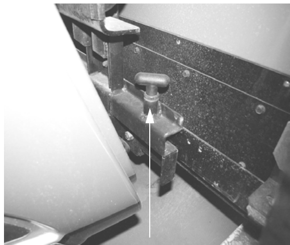
Security T-Pin (Located on the passenger side of the lower front hood bracket)
