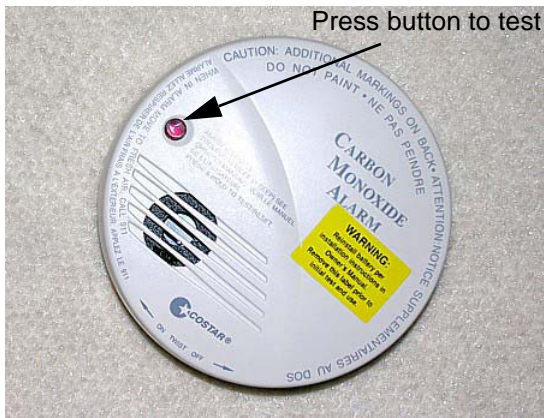
Carbon Monoxide Alarm
