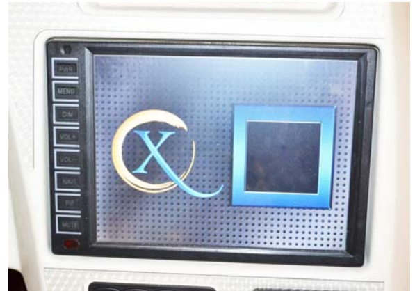
Radio/Rearview Monitor (Located on dash) -Typical View
