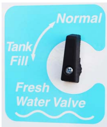
Fresh Water Valve (Located in water service center) -Typical View
