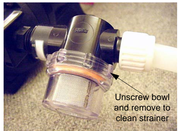
Water Pump Strainer -Typical View
