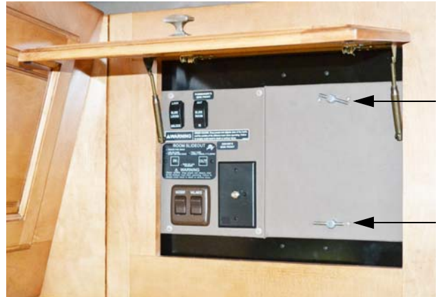
Access Panel Cover Latches Turn “counter-clockwise” to remove cover.
