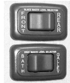
Black and Gray Waste Level Selector Switches (Located near monitor panel)
