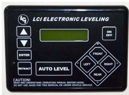
Leveling System Control Panel (Located on dash)
