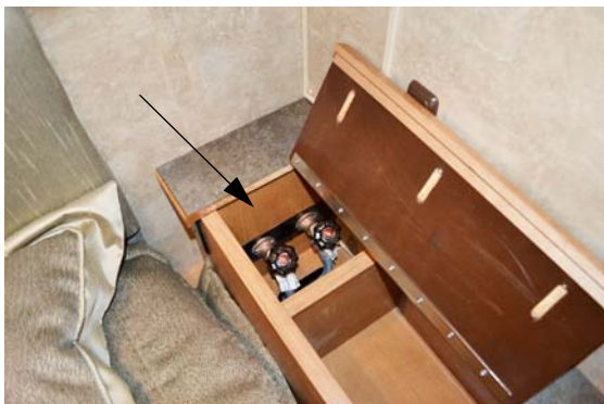
Water Supply Faucets (Located inside front nightstand)
