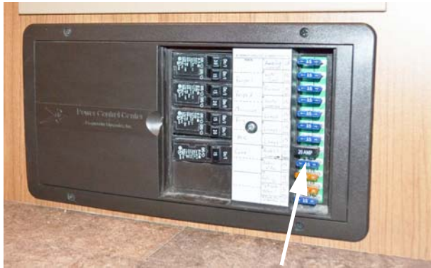
House 12-Volt Fuses (Located on the right-hand side of the Power Converter) (Models 27N and 30T) -Typical View
