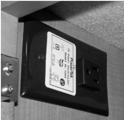
Front TV Ignition Switch Interlock -Typical View
