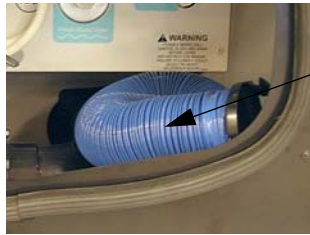
Sewage Drain Hose -Typical View
