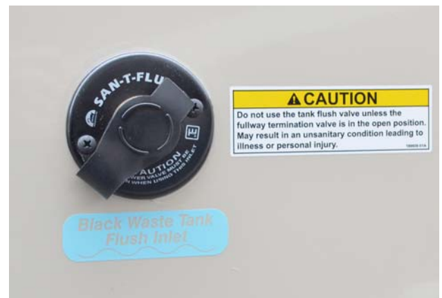
Black Waste Tank Flush Inlet (Located on left sidewall) -Typical View
