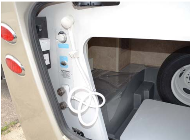
Using exterior shower to drain waterline.
