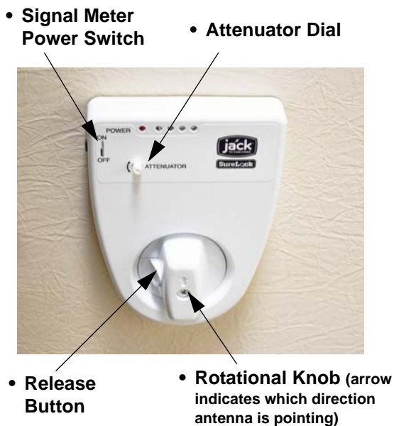
Digital Antenna Signal Meter (Located on ceiling)
