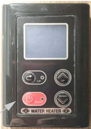
Water Heater Power Switch (Push to turn ON)
