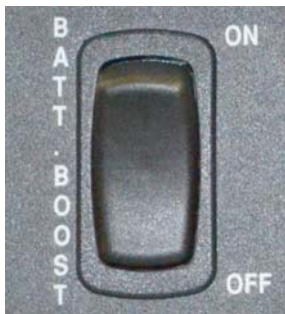
Battery Boost Switch
