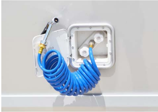
Exterior Shower/Wash Station (Typical)
