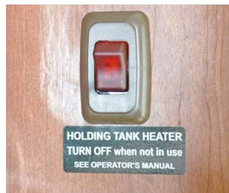
Holding Tank Heater Switch (Located near monitor panel) -Typical View
