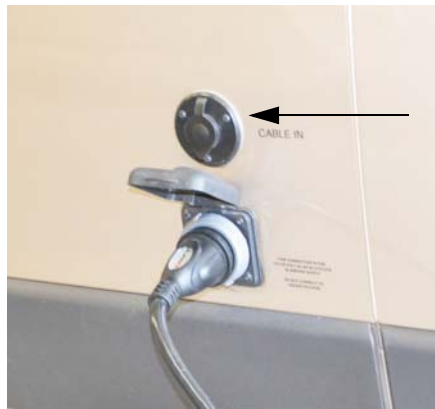
Cable TV Input Connection (Located on the left sidewall) *Model 59G shown
