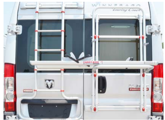
Pull straight down to lower bike rack for use. (shown in down position)
