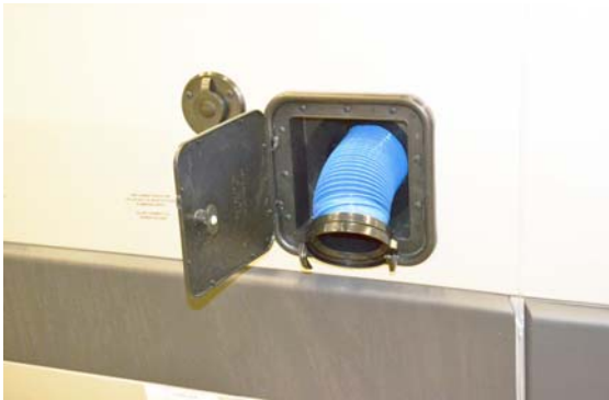
Sewage Drain Hose (Located on left sidewall) -Typical View
