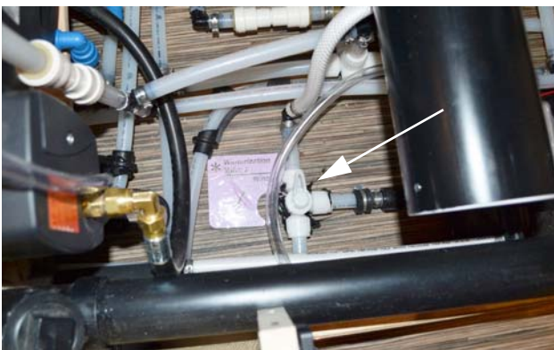
Water Heater Bypass Valve (See “Water System Drain Valve Locations” chart at the end of this section for location on your model) *Model 59K shown with bed top removed
