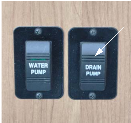
Waste Pump Switch (Located behind rear passenger side door) -Typical View
