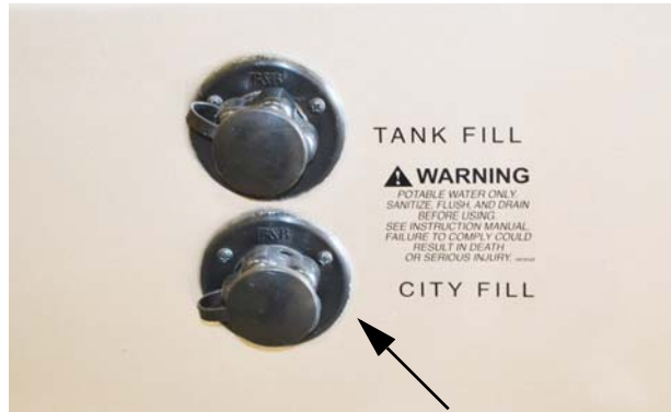
City Fill Inlet (Located on the left sidewall) -Typical View
