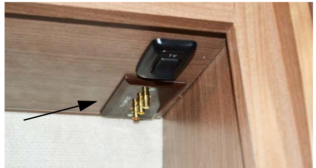
Composite Connection • Model 59G: Located in cabinet behind TV. • Model 59K: Located in overhead cabinet above TV. -Typical View
