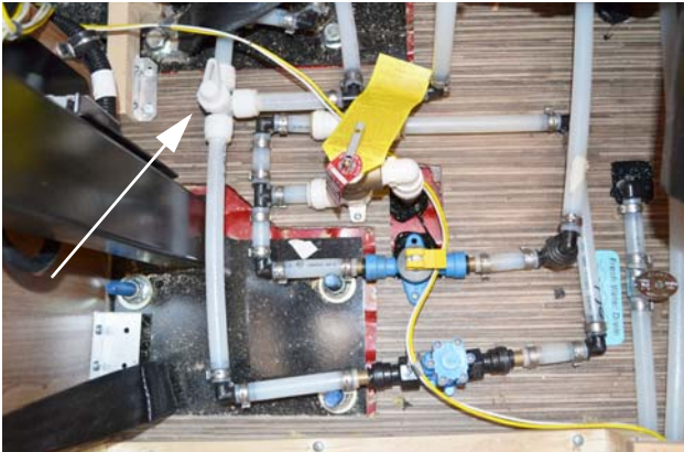
Water Heater Bypass Valve (See “Water System Drain Valve Locations” chart at the end of this section for location on your model) *Model 59G
