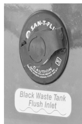
Black Waste Tank Flush Inlet (Located on left sidewall) -Typical View
