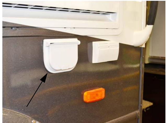
Exterior Cable TV / 12-Volt Connection (Located near entrance door) -Typical View
