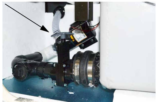
Gray Waste Tank Drain Valve (Located in driver side compartment behind rear wheel)
