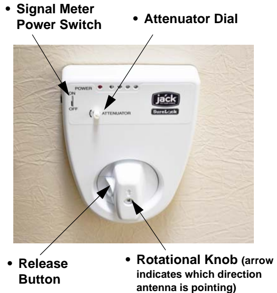
Digital Antenna Signal Meter (Located on ceiling)
