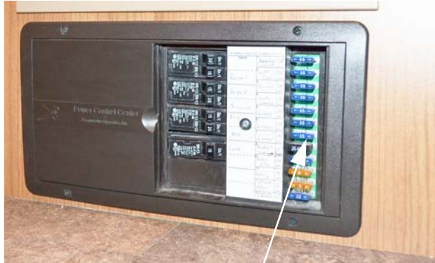
House 12-Volt Fuses (Located on the right-hand side of the power converter) -Typical View
