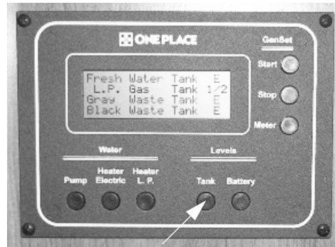
Tank Levels Switch
