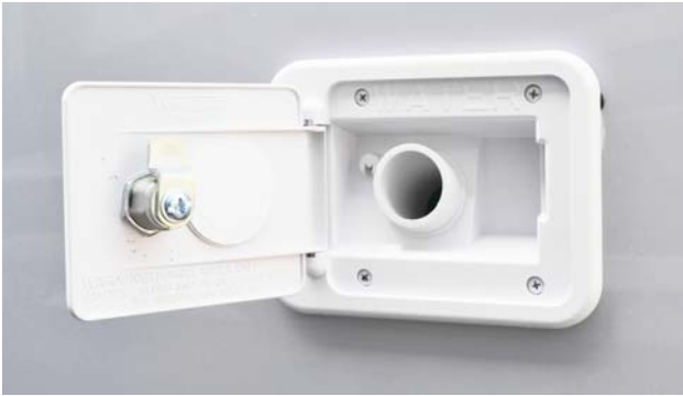
Water Tank Gravity Fill -Typical View
