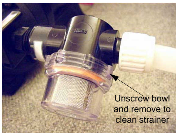
Water Pump Strainer -Typical View
