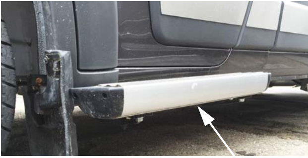
Accent LED Light Strips (Located on driver side running board) -Typical View
