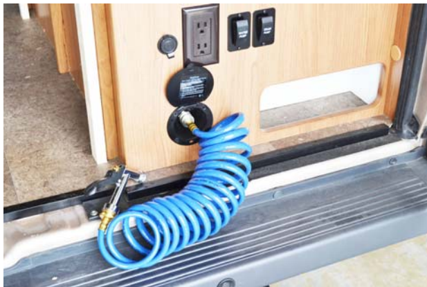
Exterior Shower/Wash Station (located behind rear passenger side door) *Model 59G shown
