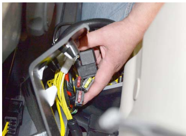
Trailer Plug and Step Fuses (Located behind plastic panel on pillar behind passenger seat)
