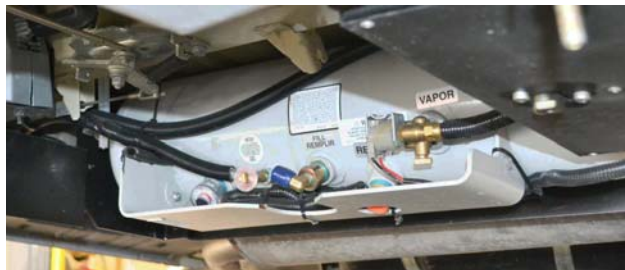
Propane Gas Tank (Located under center of coach) -Typical View
