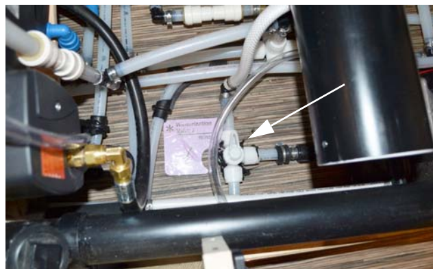
Water Heater Bypass Valve (See “Water System Drain Valve Locations” chart at the end of this section for location on your model) *Model 59K shown with bed top removed
