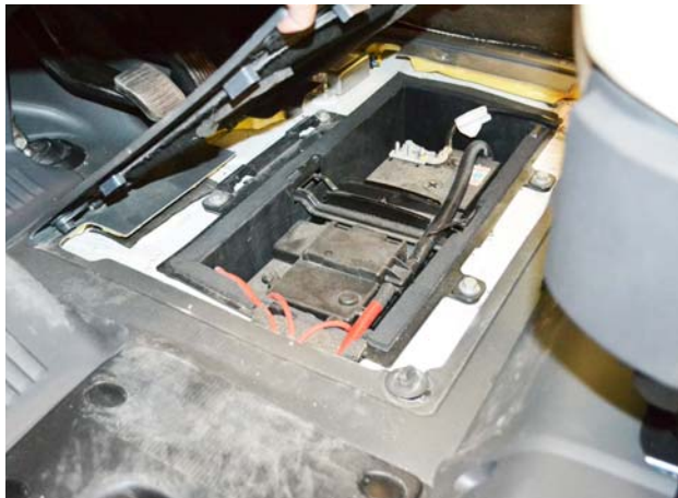
Chassis Battery Access (Located beneath driver side floor mat) -Typical View
