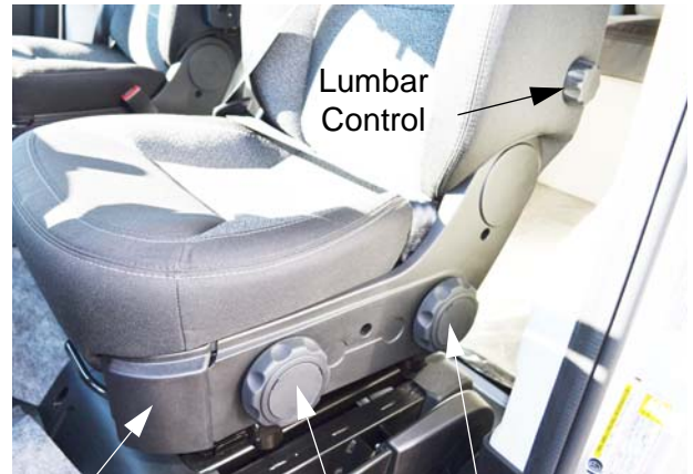
Seat Recline Front Height Control Rear Height Control Driver Seat -Typical View
