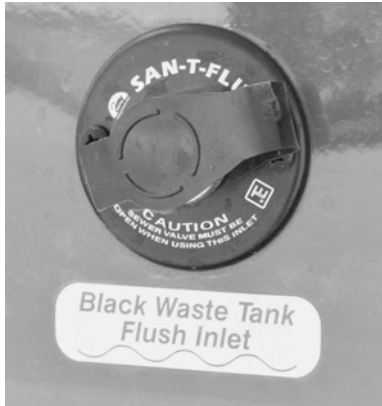
Black Waste Tank Flush Inlet (Located on left sidewall) -Typical View
