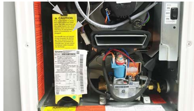
Easy Drain Lever (Located behind water heater access panel on exterior of coach)
