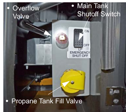
Propane Gas Access (Located in driver side compartment) -Typical View
