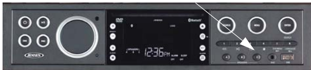
Exterior Speaker Switch “Speaker C” (Located on the interior stereo radio)
