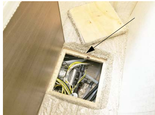
Water Pump (Located beneath removable access panel in bedroom floor on driver side front of bed) -Model 24G shown
