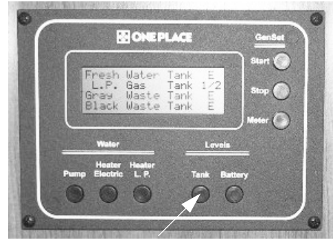
Tank Levels Switch
