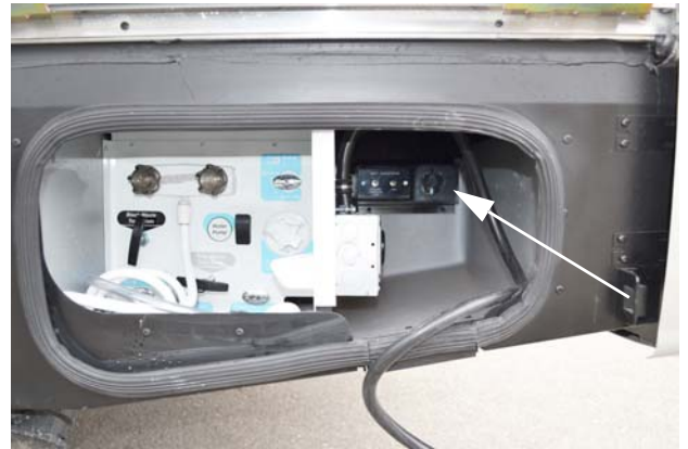
Single Solar Port (Located inside rear driver side exterior compartment)
