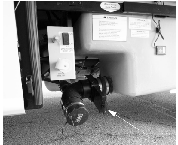
Black Waste Tank Drain Valve (Located in driver side compartment) -Typical View
