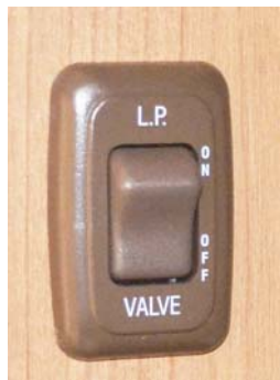
LP Tank Valve Switch
