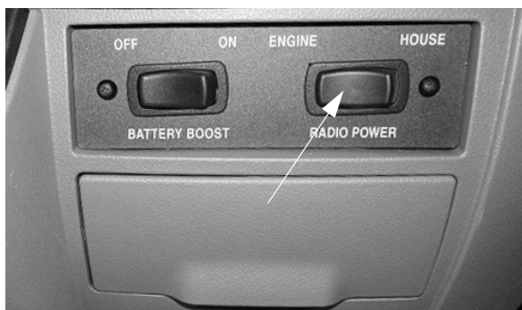
Radio Power Switch (Located on dash)
