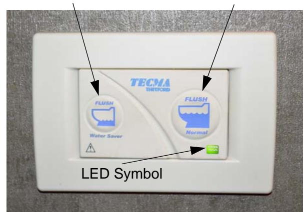
Wall Switch/Controller (Located on wall near toilet)
