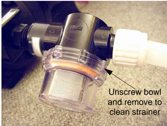
Water Pump Strainer -Typical View
