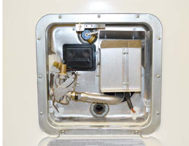
Water Heater Exterior Service Access
