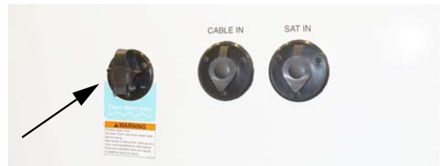
Fresh (City) Water Connection “Fresh Water Inlet” (Located on driver sidewall) -Typical View
