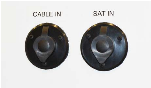
Satellite Dish and Cable TV Connections (Located on the left sidewall) -Typical View
