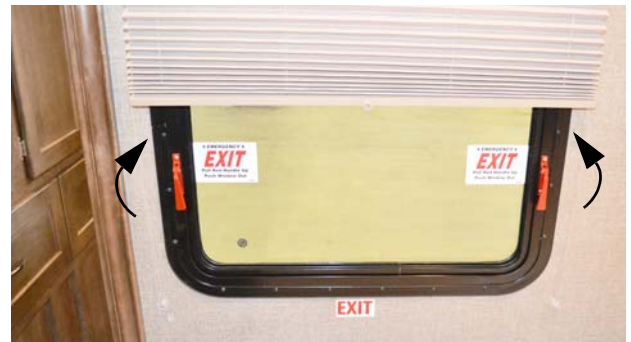
Escape Window (Lift both red safety latch handles UP and push window OUT) -Typical View
