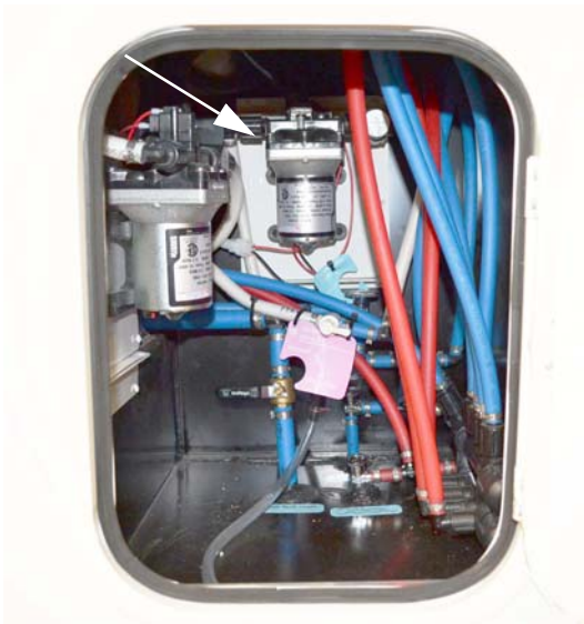
Water Pump (Located in passenger side compartment behind rear axle)
