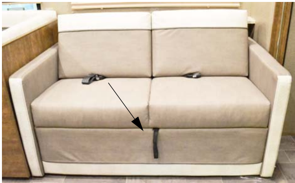
Security Latch Strap Pull strap DOWN to release security latch -Typical View
