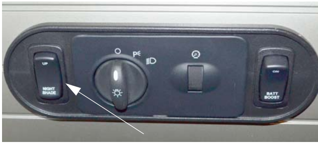
12-Volt Front Drop-Down Night Shade Switch (Located on driver side trim panel) -Typical View
