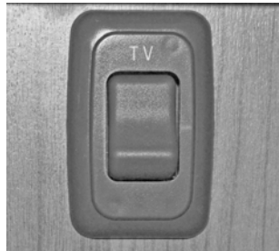
12-Volt TV Master Power Switch (Located in cabinet behind front overhead TV) -Typical View
