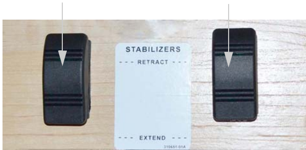
Stabilizing Jack Switches (Located inside lower passenger rear compartment) -Typical View
