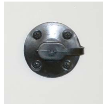
Single Solar Port (Located in power cord compartment)
