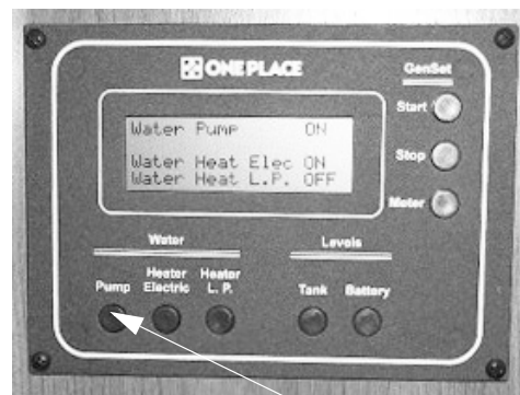
Water Pump Switch
