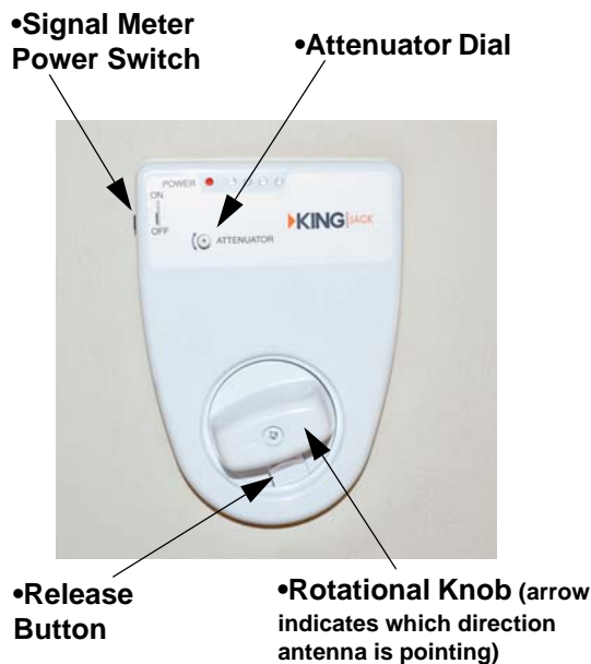
Digital Antenna Signal Meter (Located on ceiling)
