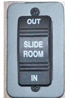
Slideout Switch (Your motorhome may have one or more slideout switches depending on model, options, and available equipment) -Typical View
