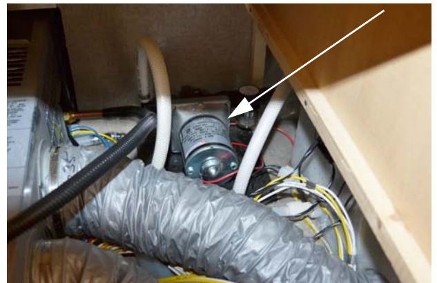
Water Pump • Model 23T - located beneath galley (remove panel to access) -Typical View
