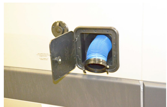
Sewage Drain Hose (Located on left sidewall) -Typical View
