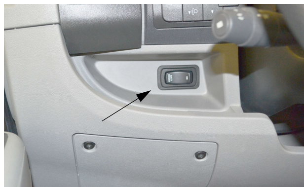
Battery Boost Switch (Located on lower dash area)
