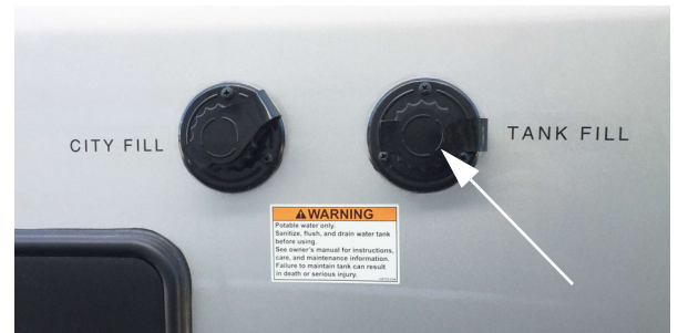
Tank Fill Inlet (Located on the left or right sidewall, depending on model) *Model 59K shown
