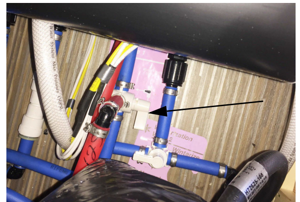
Winterization Valve 1 (Water Heater Bypass Valve) (See “Water System Drain Valve Locations” chart at the end of this section for location on your model) *Model 59K shown
