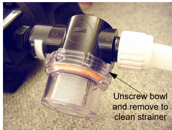
Water Pump Strainer -Typical View
