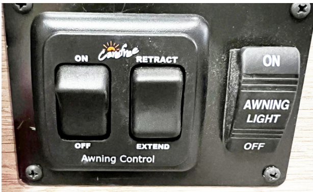
Power Awning control switches and Awning Light Switch (Located near sliding entrance door) -Typical View
