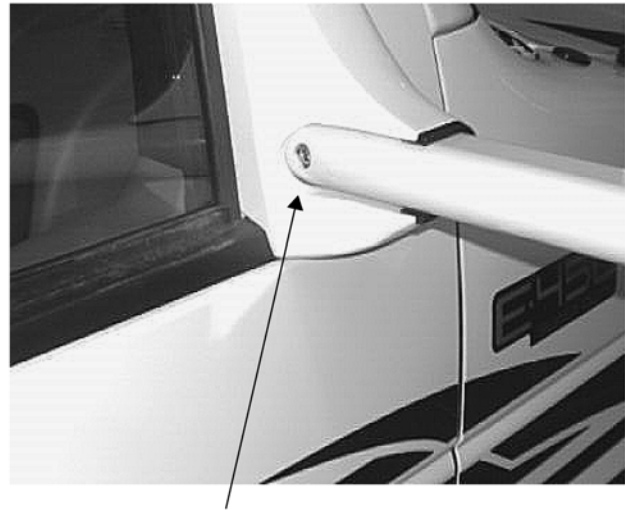
Mirror Arm Tension Adjustment Screw
