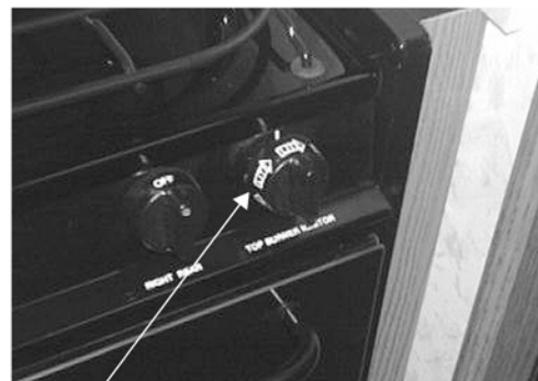
Rotate Ignitor Knob while Burner Knob is in LITE position.
