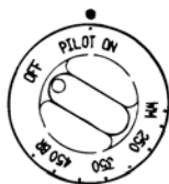
Oven Control Knob in "PILOT ON" position
