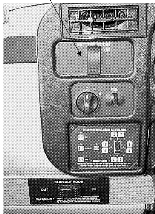
Battery Boost Switch
