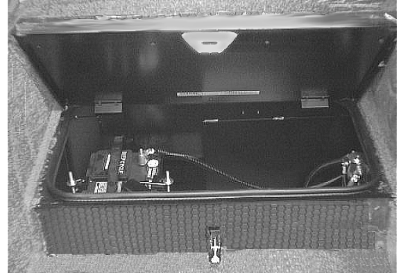
House Battery in Top Entrance Step
