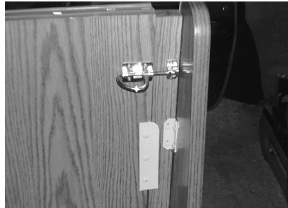
Dinette Seatback Latch (Remove cushion and unbolt to fold down)
