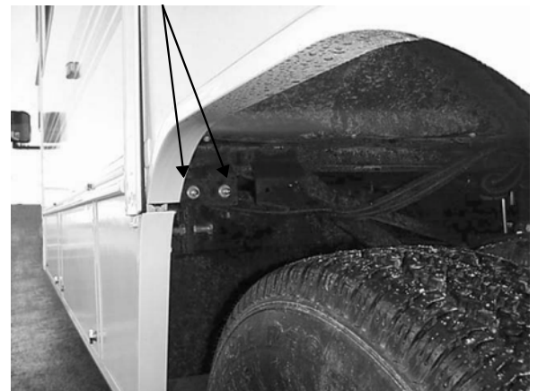
Rear Helper Spring Air Valves located inside left rear wheelwell
