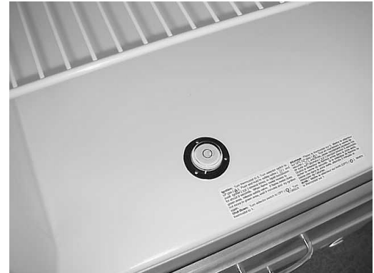
Place bubble level in bottom of refrigerator
