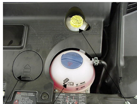
Oil Fill Access
