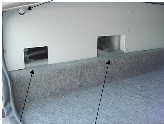
Winterizing Valve and Water Tank Drain Valve Access in RH Storage Compartment
