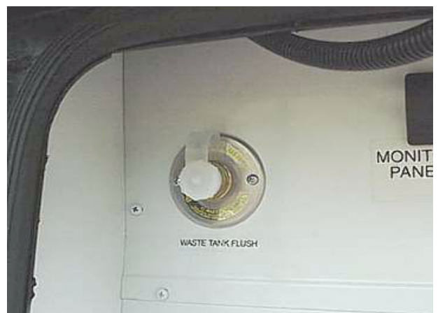
Black Tank Flush Inlet
