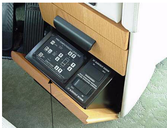
Automatic Leveling System Control Panel
