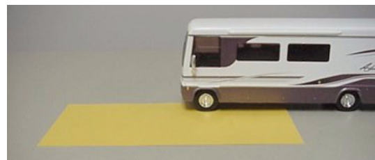
Weighing Left Front 'Corner'
