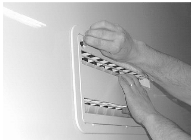
Turn latches open with coin
