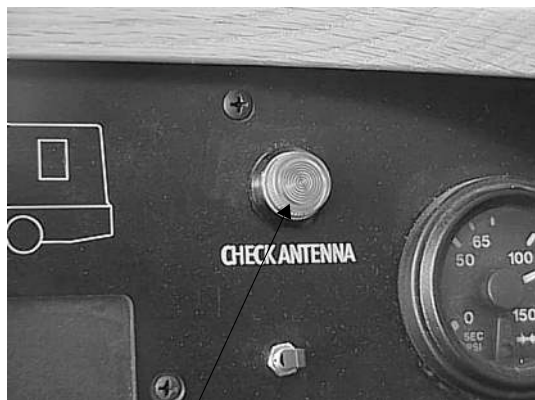
“Check Antenna” Light
