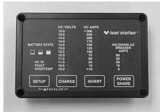
Inverter Charger Control Panel
