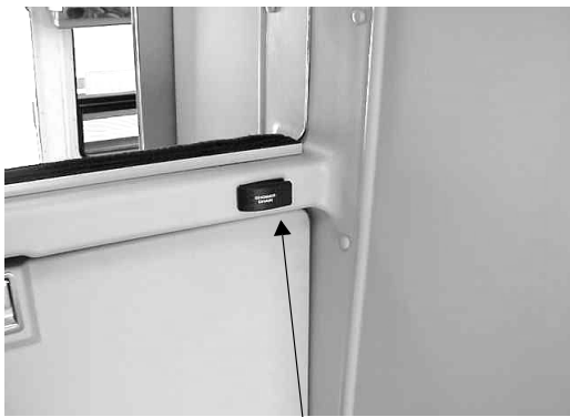
Shower Drain Pump Switch
