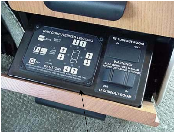
Leveling System Control Panel
