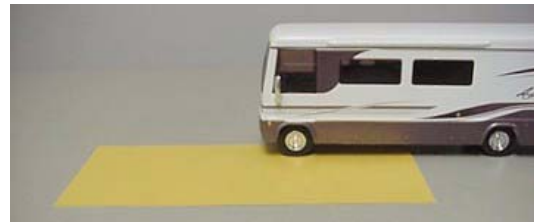
Weighing Left Front 'Corner'
