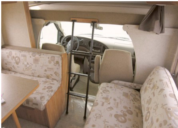
Front Overhead Bunk Shown with bunk sections and ladder in use position
