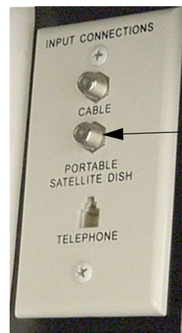
Exterior Connection for Satellite Dishes (In Water Center Compartment)
