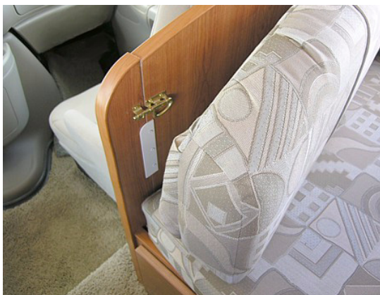
Dinette Seatback Latch (Remove cushion and unbolt to fold down)
