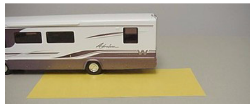
Weighing Left Rear ‘Corner’
