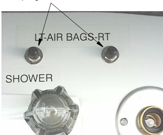
Rear Air Spring Fill Valves located inside water center
