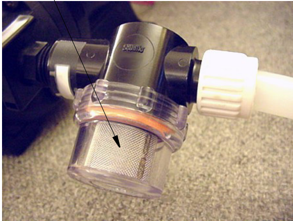
Water Pump Strainer
