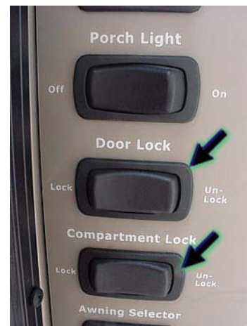
Power Door Locks on entry switch panel
