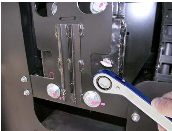
Crank the Slideout Retract Bolt with the Ratchet Wrench provided.
