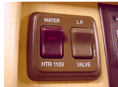
Main Tank Valve on OnePlace Panel
