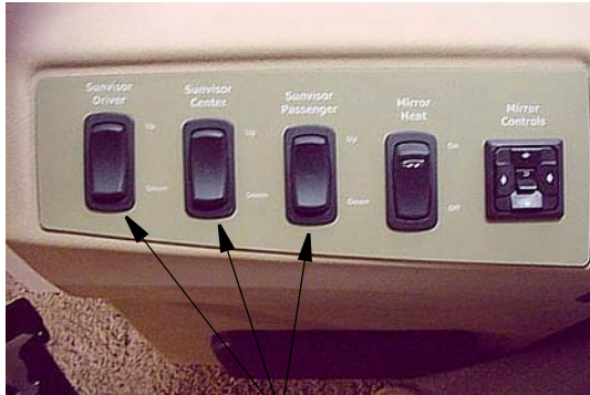
Driver Side Sunvisor Switches (center visor not equipped on models 40FD & 40TD)
