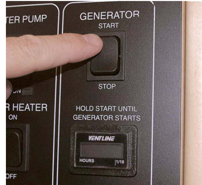
Generator Switch and Hourmeter
