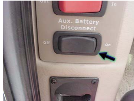
Aux. Battery Disconnect Switch (Near entrance door)
