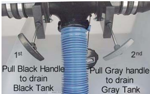
Holding Tank Valves (Typical)
