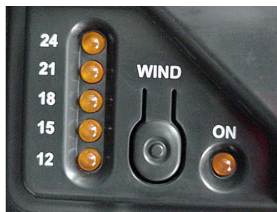
Wind Sensor Control Switch and Indicators on Control Box
