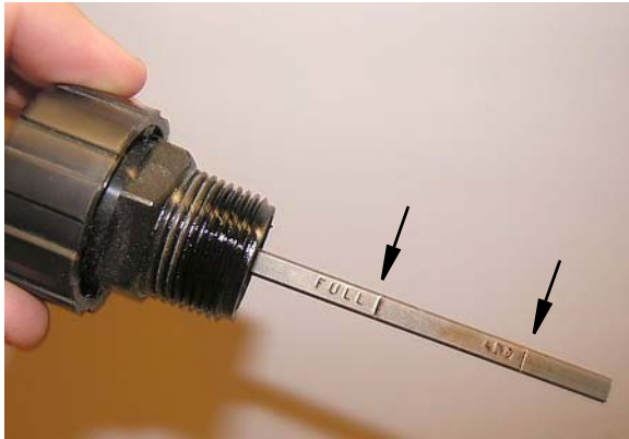
Hydraulic Fluid Dipstick HWH System Pump (F38J Model Only)
