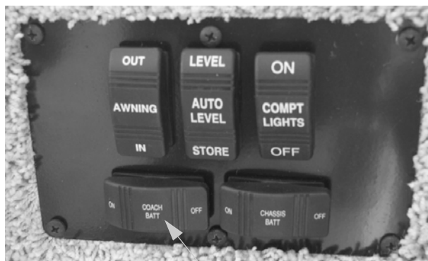
Auxiliary Battery Switch - Typical (Near Entrance Door)
