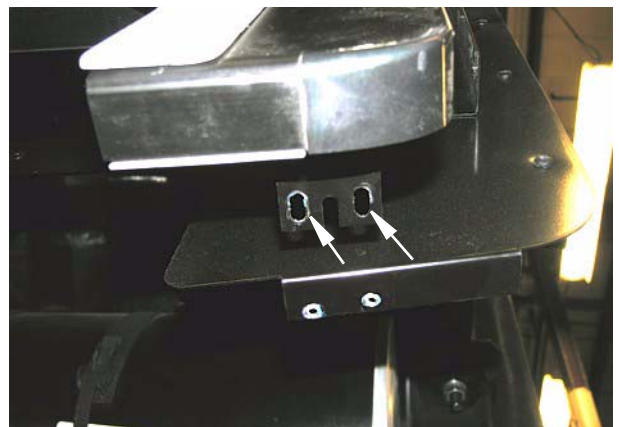
Remove 2 screws in lower rear edge of grill panel shown, then swing hinged panel upward.
