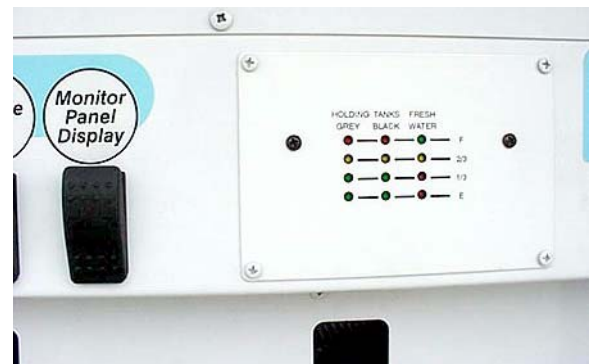
Water Center Tank Level Monitor -Typical
