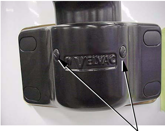
Unscrew protective caps and loosen Allen head set screws to pivot mirror arm. (Torque screws to 75-100 in./lbs.)
