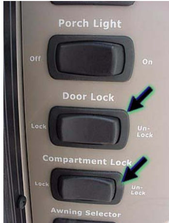
Power Door Locks on entry switch panel
