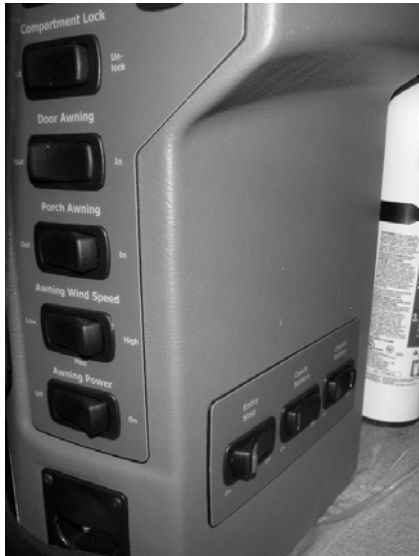
Awning Control Switches - Typical View (Located near entrance door)
