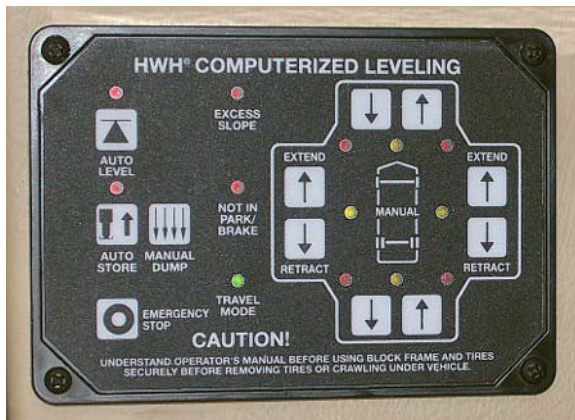
Leveling System Control Panel
