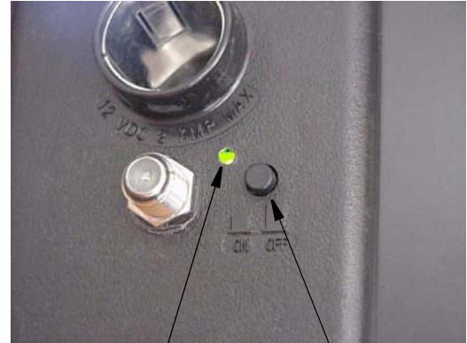
Power indicator glows when signal amplifier is active
