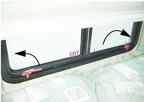
Escape Window (Lift both red safety latch handles UP and push window OUT) -Typical View
