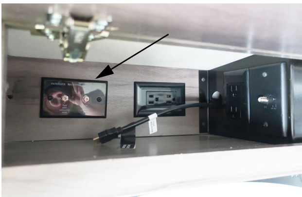
Interior Connection for Satellite Dish -Typical View
