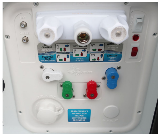
Sanitize configuration -Typical View
