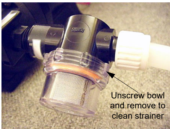
Water Pump Strainer -Typical View
