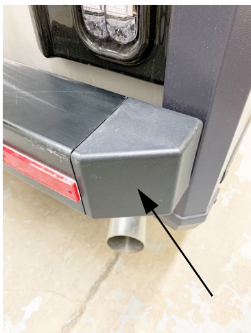
Passenger side blind spot sensor location. Do not paint or cover this block. -Typical View
