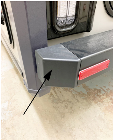
Driver side blind spot sensor location. Do not paint or cover this block. -Typical View
