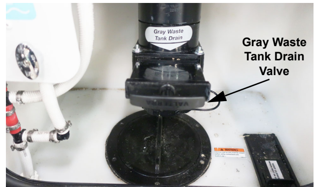
Sewage Drain outlet (Located inside the service center on the drivers side) -Typical View
