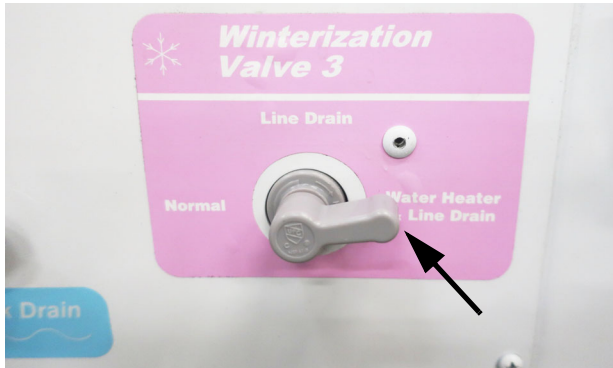
Winterization Valve 3 turned to the “Water Heater and Line Drain” position. -Typical View
