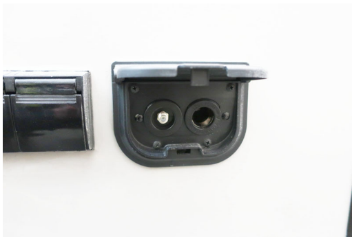
Interior Connection for Satellite Dish (Located on the passenger sidewall) -Typical View
