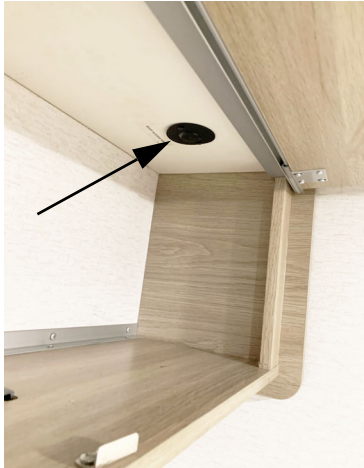
Roof Access Port (Located inside rear overhead cabinet). -Typical View
