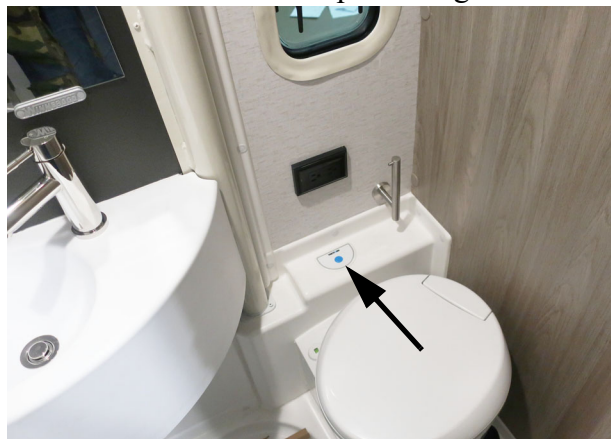
Toilet flush button. Hold until water stops flowing. Model 622A shown. -Typical View
