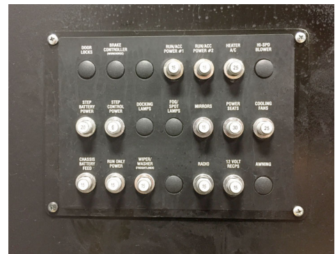
Automotive Circuit Breakers (push to reset) • Breakers are labeled for components equipped
