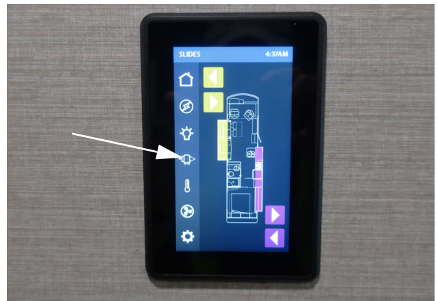
Slideout Switch (Located on Multiplex Monitor Panel) -Typical View
