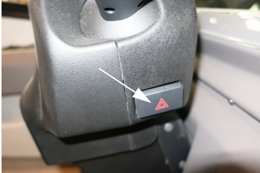
Hazard Warning Flashers (Typical View - your motorhome may differ depending on model)
