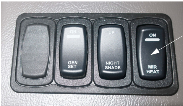
Mirror Heat Switch (Located on driver side trim panel) -Typical View
