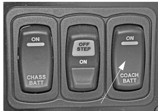
House/Coach Battery Disconnect Switch (Located near entrance door) -Typical View
