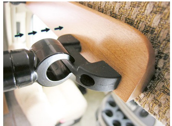
Attaching Bunk Ladder
