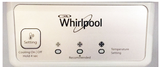
Cooling ON/OFF Press and Hold for 4 seconds
