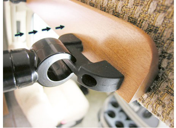
Attaching Bunk Ladder
