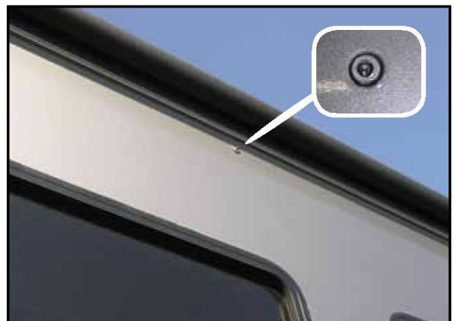
The Slideout Lock Drain Line (inset) is located near the top of the exterior slideout room.
